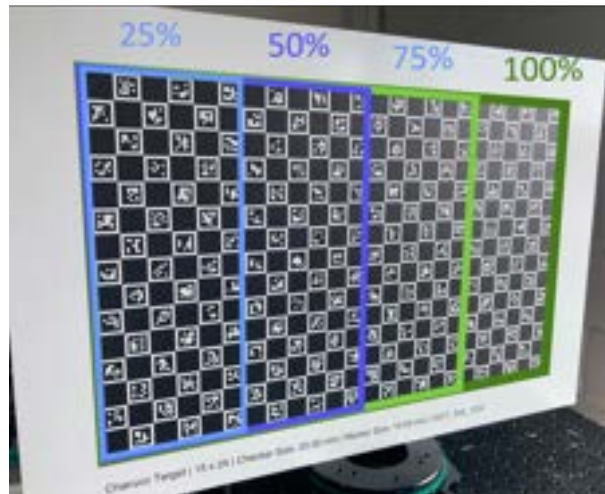
Figure 14: Illustration of visible/used markers for valid calibration data
