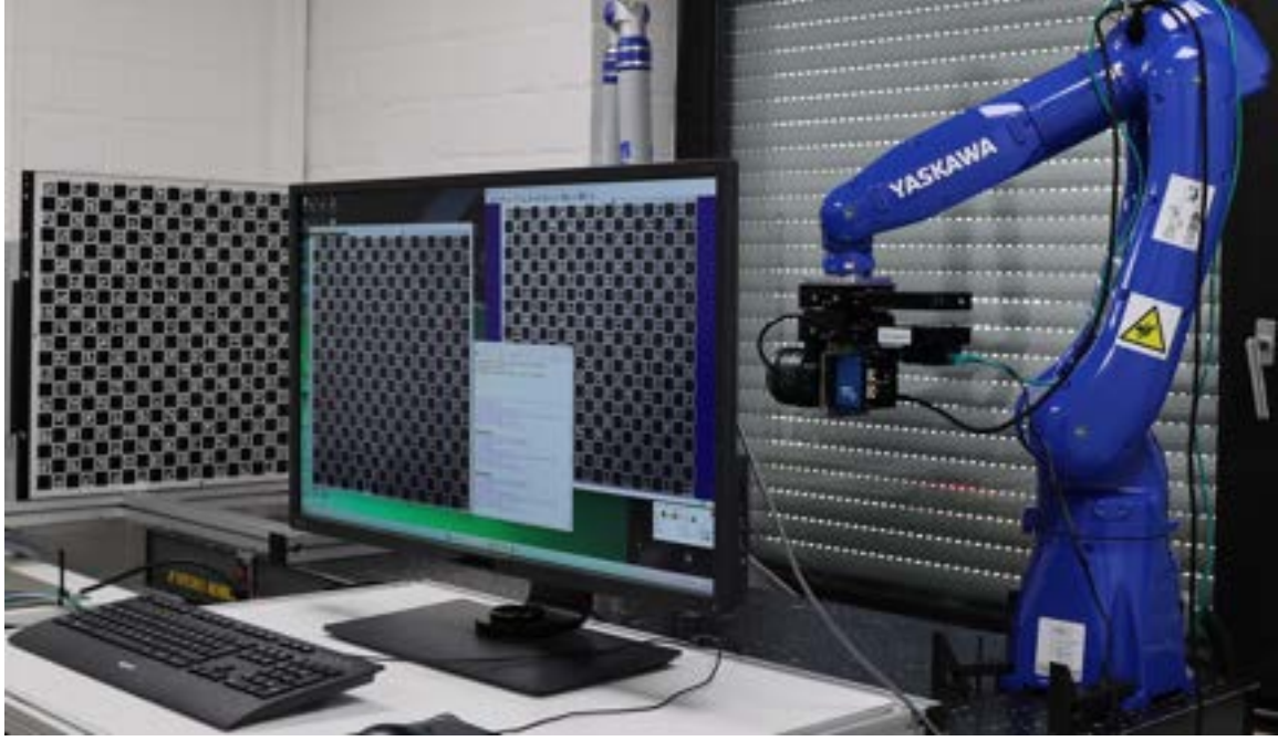
Figure 6: Complete calibration setup with a large customized ChArUco target and live image of the calibration process
